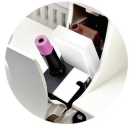
Advanced Radio Frequency (RF) technology automatically detects the latex reagent information, instead of manual scanning, which makes it more convenient.
